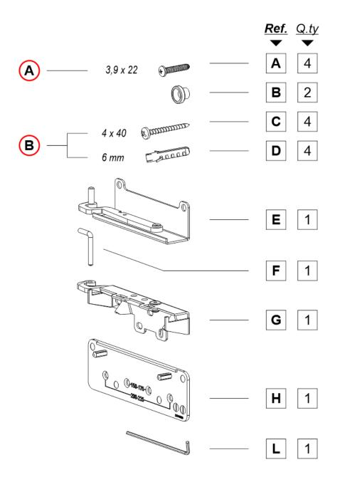
A) - For door frame / elevator car wall fixing
