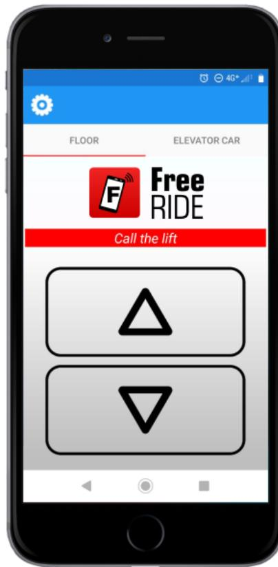
Restart the FreeRIDE application. The layout of the button panel is displayed on the smartphone screen.
